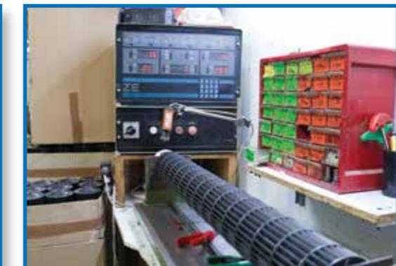
Ultrasonic welding machines for plastic fans production and fan balancing machines for precise parts production.
