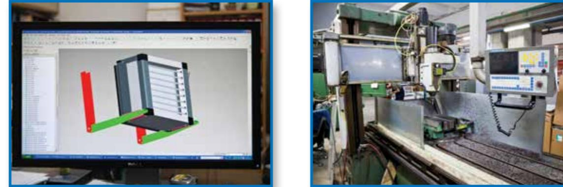
PRO Engineer Software station for MOULD design connected with a 4 AXIS CNC mill with a long up to 3 meters table for big Moulds production.
