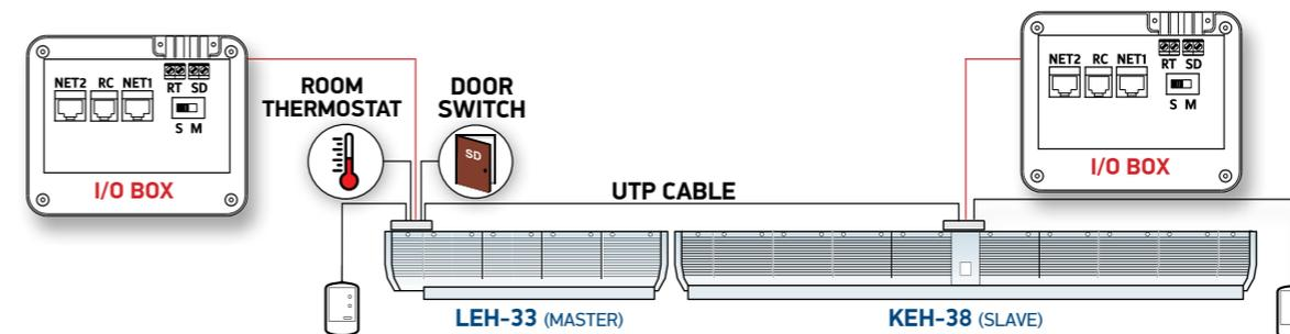
**OLEFINI** Heated Air Curtains (*Electrical or water*) have a wired-infrared remote control, allowing to switch **ON-OFF** the device, to change fan speed, to change heating level (**HEAT POWER**) or to control the hot water solenoid valve (**WATER VALVE**) depending on the way of heating.
