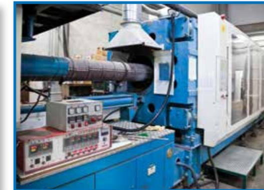
CNC Automated Injection machines production line for plastic parts, capable of producing parts weighting from 10 gr up to 6.5 kgr.
